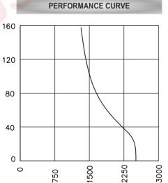
Air volume —→ [M<sup>3</sup>/hr] Conversion: 100pa ≈ 0.4" H20 100m<sup>3</sup>/hr ≈ 60cfm
